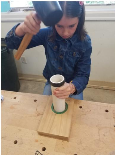
Jordan presses the screen into the board, rolls the PVC pipe a couple times to properly form the screen, and pushes it out the bottom of the hole.
