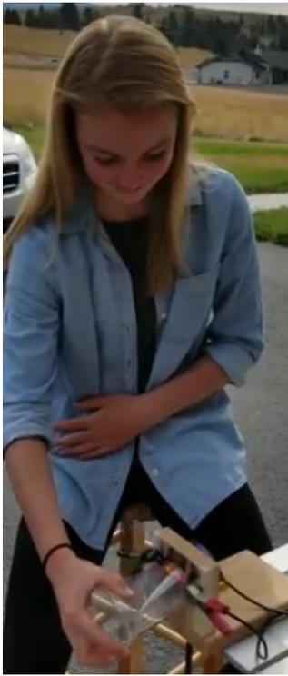
Dylan cuts the bottom from each screened cup using an 18 gauge nichrome wire jig. (Cut the cups outside and don't breathe the nasty fumes of the burning plastic.) We attached the clamps from a manual battery charger **on the 6 volt setting** to the two bolts which hold the nichrome wire.
