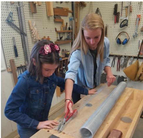
Dylan and Jordan cut #8 hardware cloth into 3½ inch strips (89mm). (We suggest that you use a 24" length which makes 6 screen blanks. Cutting more than 6 layers of screen at one time is difficult.)
